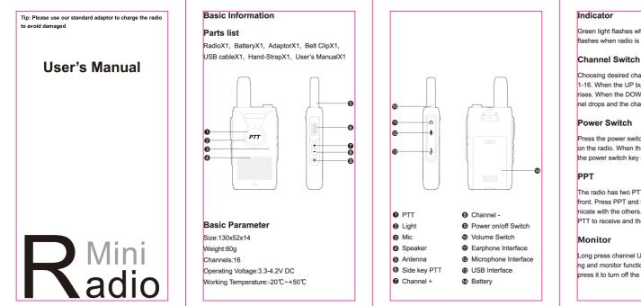
Green light flashes when radio is receiving. Red light flashes when radio is transmitting.
